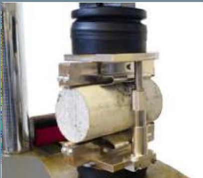
Splitting on concrete
