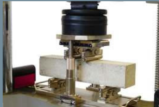
Flexure on concrete
